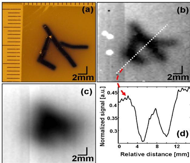
**Fig. 2** Cross-sectional UOT images of an optically absorptive patterned object. (a) Photograph of the target. (b) UOT image based on change in speckle contrast. (c) Image based on light intensity. (d) 1-D profile along the cut in.
